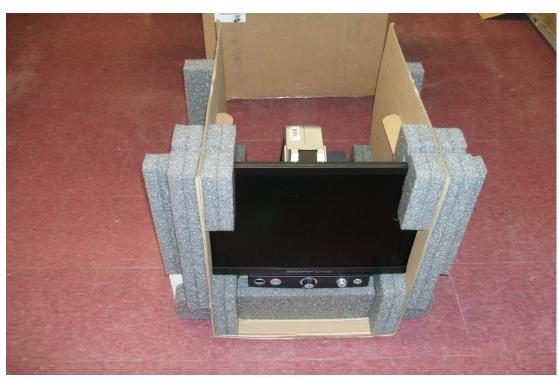
3.Open packing and lift to table that unit will be used on. \*\*\*Important\*\*\* Note hand placement for lifting so as not to damge unit's tray or camera.
