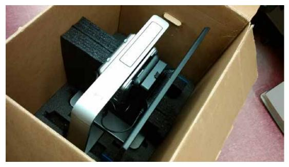
3. Lift the CCTV out of the box using the black handle.
