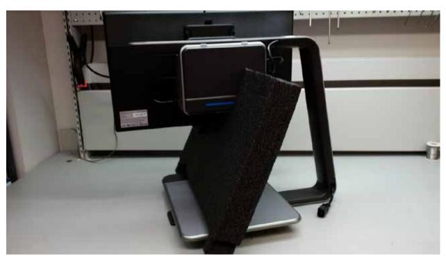
6. Insert power supply cord into cord coming from support arm. Plug into the wall.
