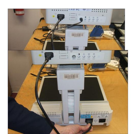
2. Remove the monitor out from the bottom unit (piece with moveable tray) by raising it out of position.
